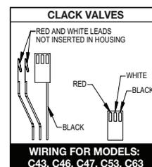
The 22 gauge wire crimp terminals are Molex Series 41572 or 40445. The housing connector is Molex Series 2695 White Housing, P/N 22-01-3037. The housing connector diagram shows the proper installation of the RED, WHITE, and BLACK wires for CustomCare control valves.
